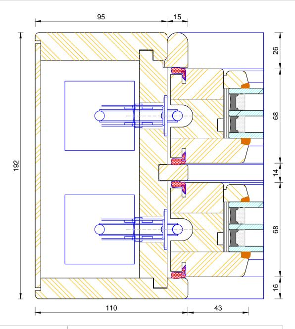
Contemporary Sliding Sash Cords & Weights Triple Glazed - Frame & Sash Jamb (Standard)
